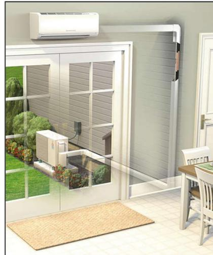
An illustration of a ductless mini-split system.
